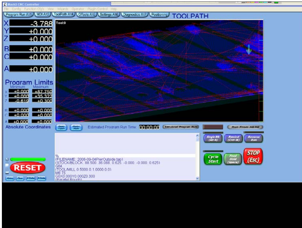
6 axis router screen 2 showing coordinate limits for the cut file.
