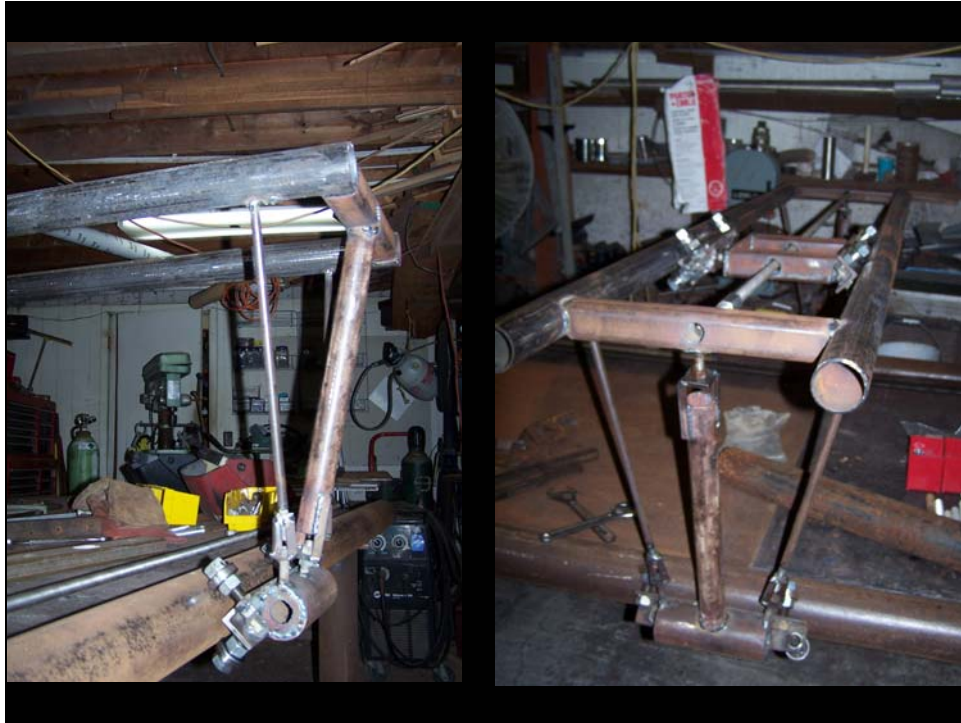
X & y axes tension struts to preload the x to the pipe rails, and adjustable to calibrate
