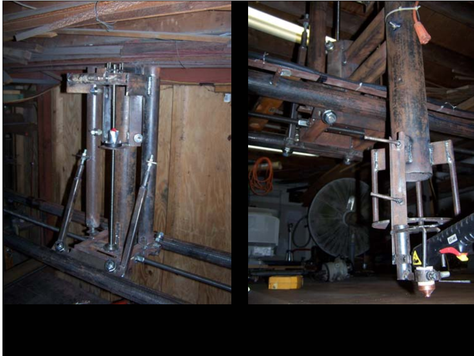
Z-axis – adjustable for vertical alignment.
