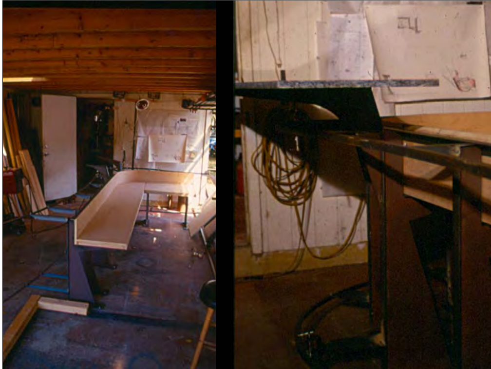
Steel Frame, CNC plasma cut (outsourced). Rolled angles for top & bot curves (outsourced) welded angled. White maple. Top is recycled, blue pearl granite stone from existing building. Allen: Masonry Chapter, Stone section.
