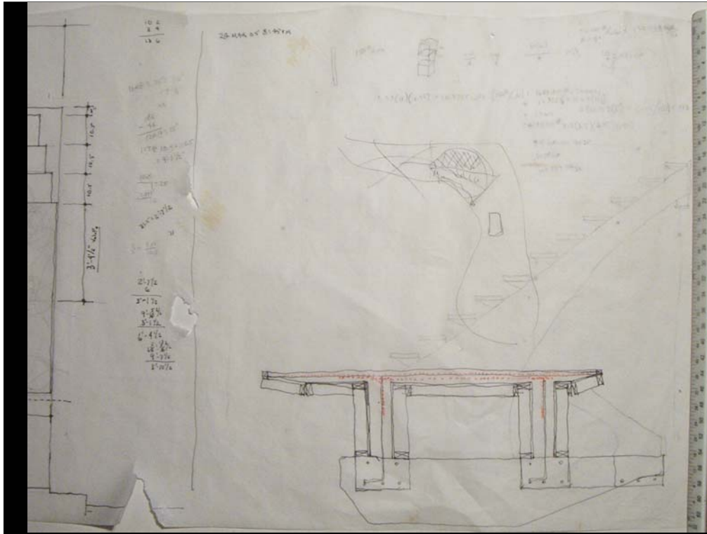
Formwork concept defined to ensure/allow it all to be removed afterward.
