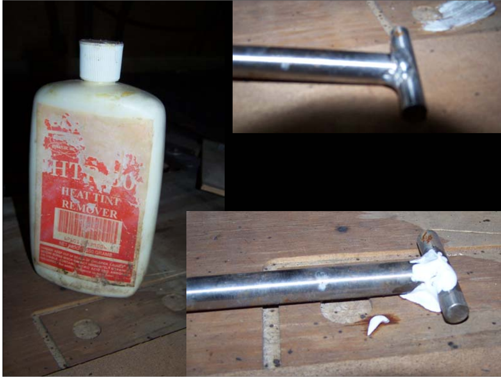
Acid based cleaner to remove heat tint produces when MIG welded.
