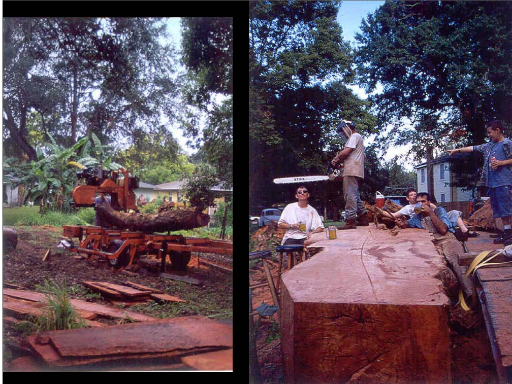
Wood mill John Kinary with his portable bandsaw mill could cut up to 24" diameter, and spent a full 9 hours milling just the branches (some of which were even too big) and could not even touch the trunk. Right: success in getting the top half of the trunk onto the trailer to take it for milling.
