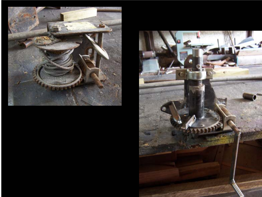
Process photos, before, during. The small angles are the stops which regulate how far the opener can turn.
